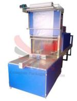
Fully automatic shrink-packaging machine including web sealer and shrink tunnel which can feed products, collating, seal and cut film and shrink film bag automatically. The machine is widely used in food, pharmaceutical, cosmetics, printing, hardware, and other industry. The machine can collate bottles (round or square), cans, gable cartons, and tetra cartons automatically. The machine can connect filling machine or labelling machine to make production line unmanned.
